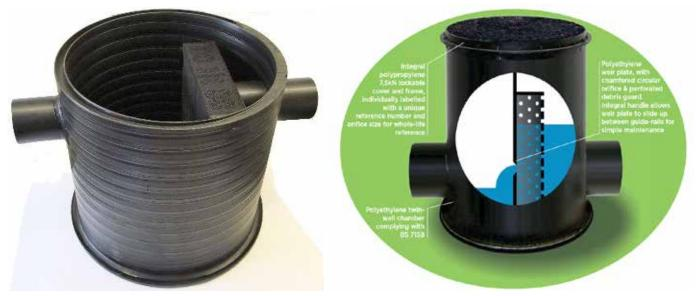
Figure 7 Example protected orifice flow controls with removable screen box (for cleaning) and with removable weir plate and perforated debris guard (for cleaning)
